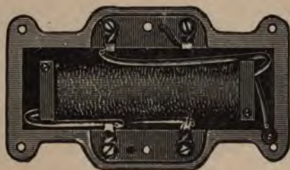
FIG. 7.—Induction coil mounted in the base of transmitter arm, showing wiring connections.
